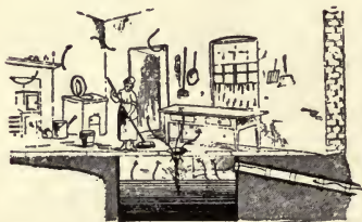
Fig. 633. Dish stone in scullery untrapped, and opening direct into a rain water tank, with overflow into drain.
